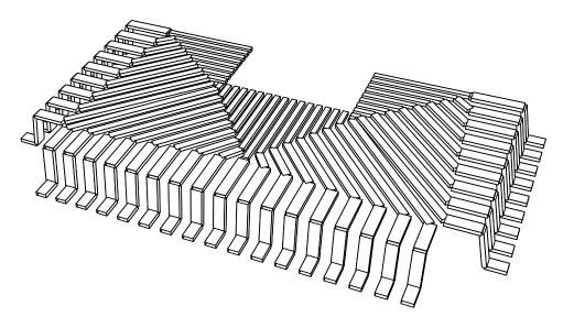
Figure 8: Thirty-Five Pins of a 68 pin Cerquad Package
